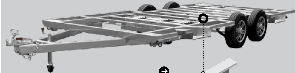
JAYCO PRESSED STEEL C-SECTION (PSC) PSC floor members are lighter than conventional box section steel, 300% stronger and resist bending by 175%.
