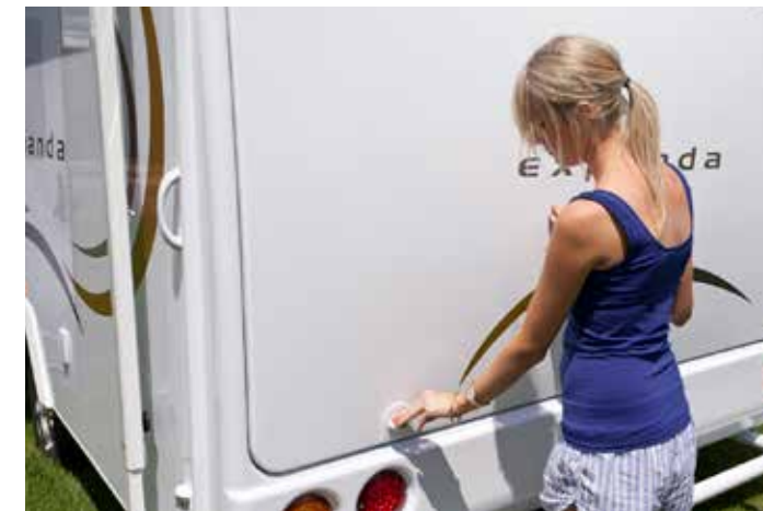
Step 1: Unlock bed end clip
