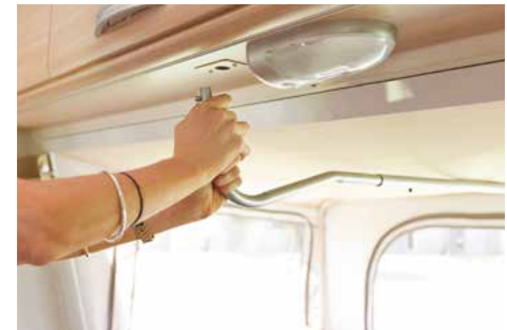
Step 4: Insert Roof Bar
