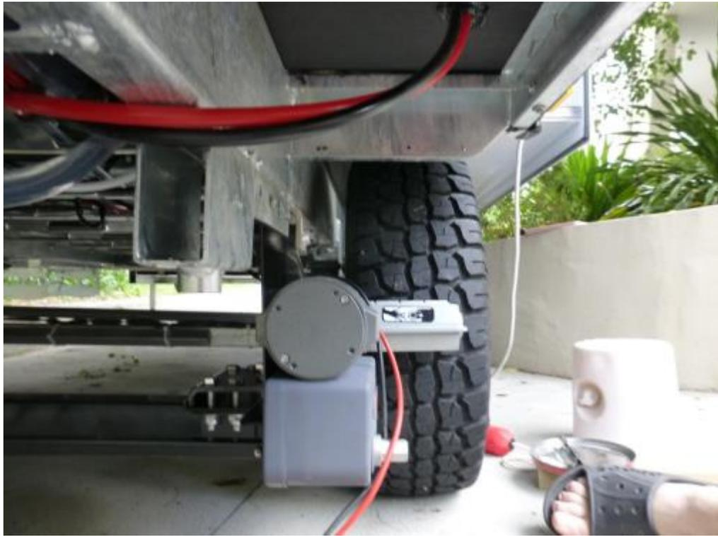
This setup gets the movers to exactly the right height - so that the drive wheel is centred on the wheel.
