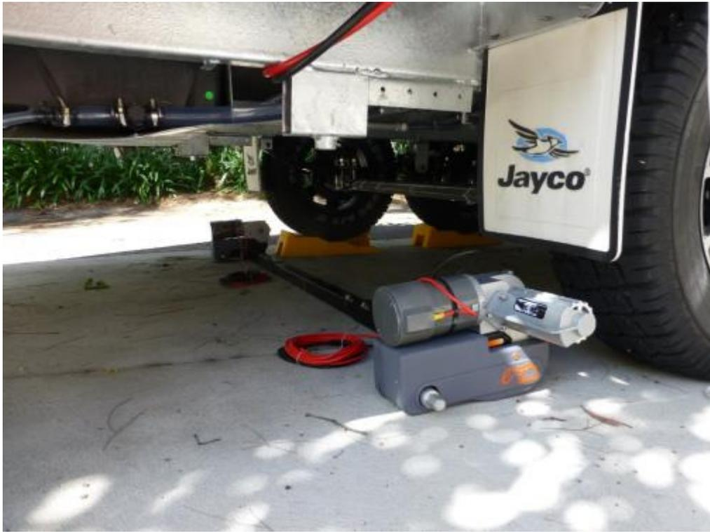
On the rear wheels you will have to remove the mudflaps and cut a few inches off as the drive will get in the way of the mudflap.
