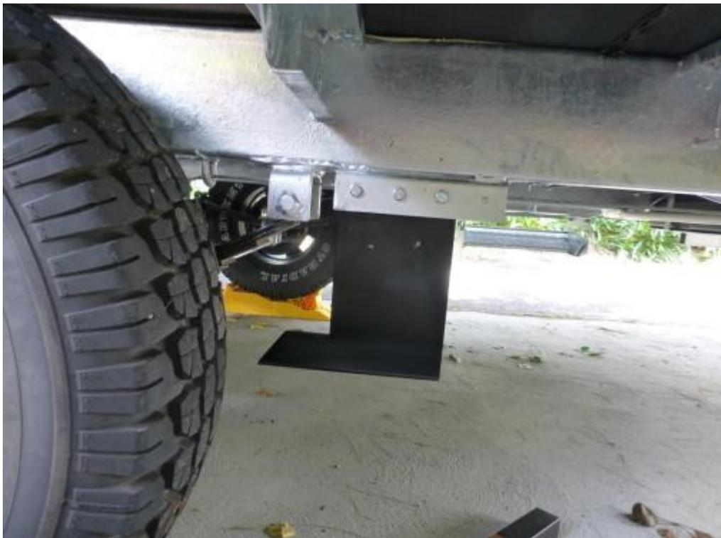
Bolt the mounting plates on to the chassis bracket
